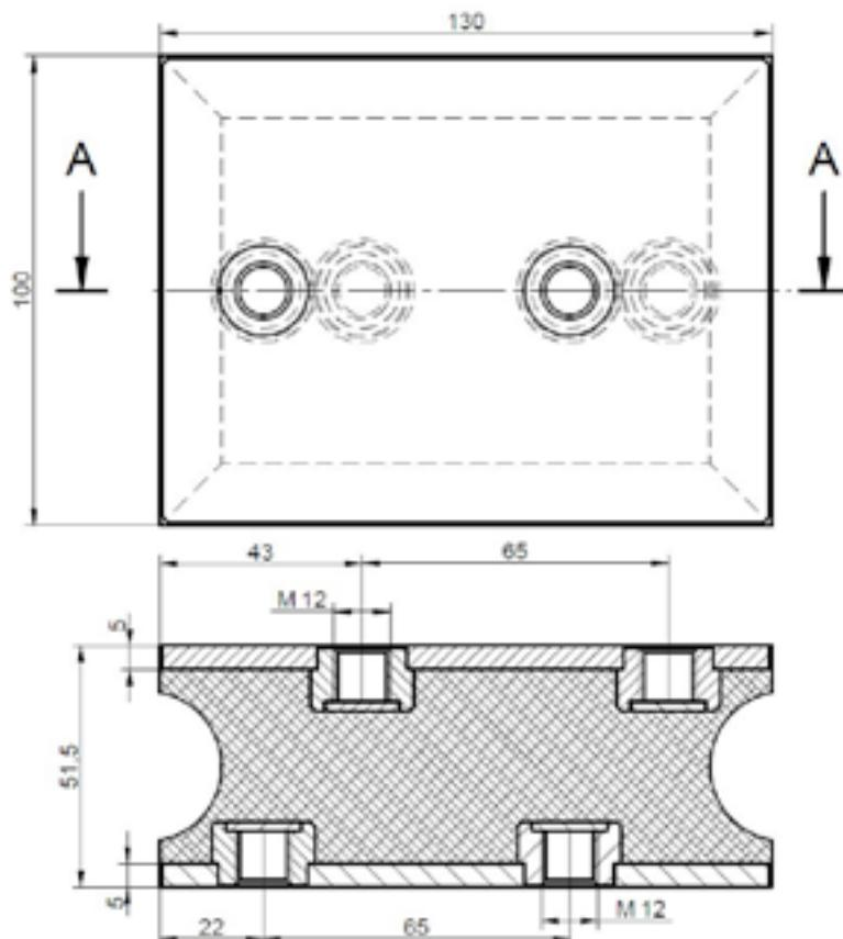
**ELASTO BT SCHIENEN / ELASTO BT SANDWICH MOUNTS**
