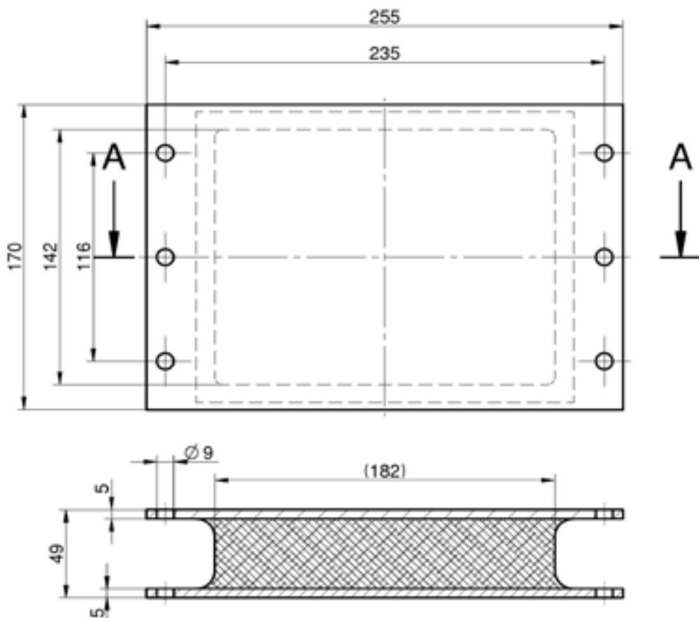
**ELASTO BT SCHIENEN / ELASTO BT SANDWICH MOUNTS**
