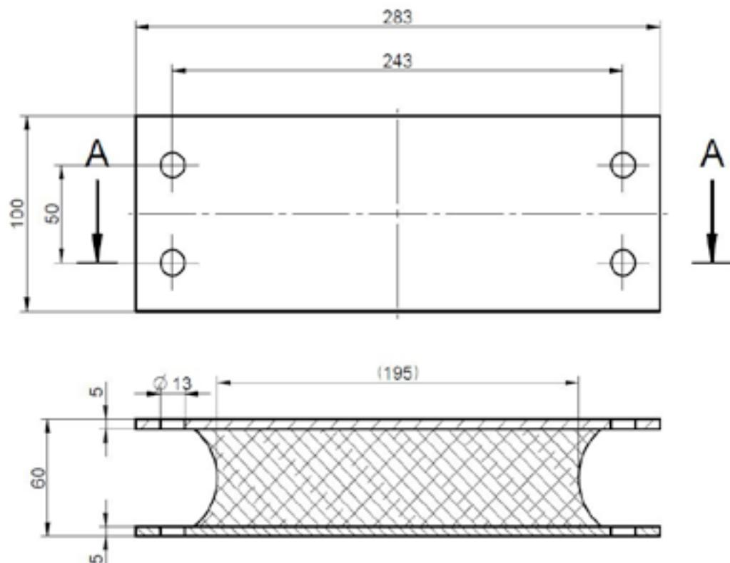
**ELASTO BT SCHIENEN / ELASTO BT SANDWICH MOUNTS**
