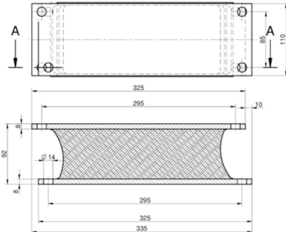
**ELASTO BT SCHIENEN / ELASTO BT SANDWICH MOUNTS**
